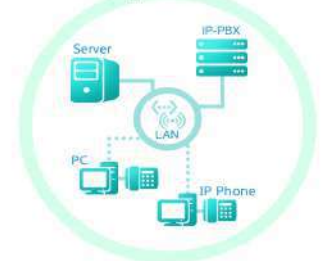
A company office using an IP-PBX
